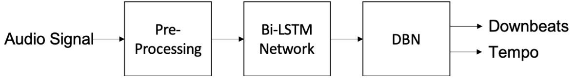
Figure 5.4: Flowchart of downbeat tracking algorithm.
