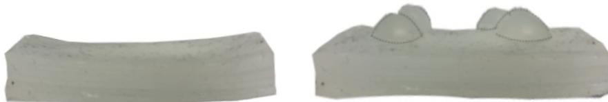
Figure 7.2: Demonstration of VPU in deflated (left) and inflated (right) states. Inflated air cells are lightly outlined for clarity.
